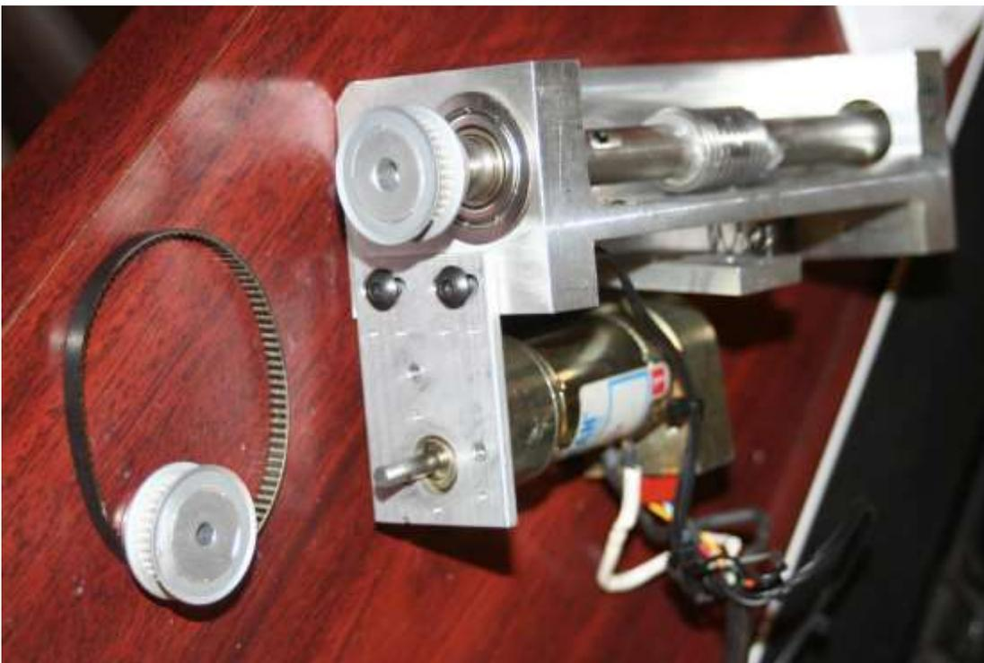
The old motor is removed and the Sitech motor fits perfectly in its place.
