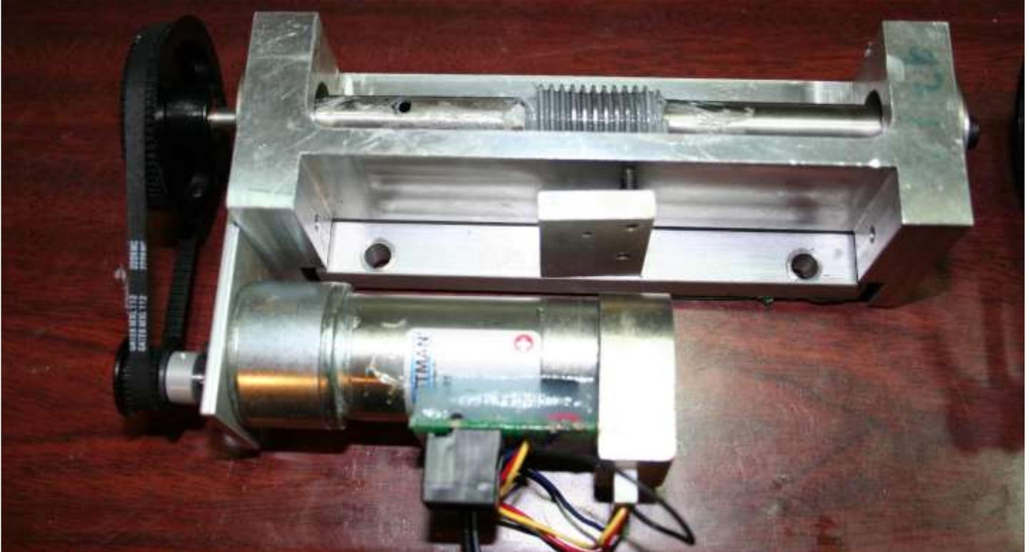
Originally I thought I would change both the ALT and Az to the 3:1 gear reductions belts and pulleys however I found out the 72 tooth pulley would not fit in the Base without major modification of the Base. And as the Az worked with the original pulleys I opted to only use the 2:1 pulleys and belts for the Az. The Sitech controller allows for different ratios for different axis so I stayed with the 3:1 ratio on the Alt axis.
