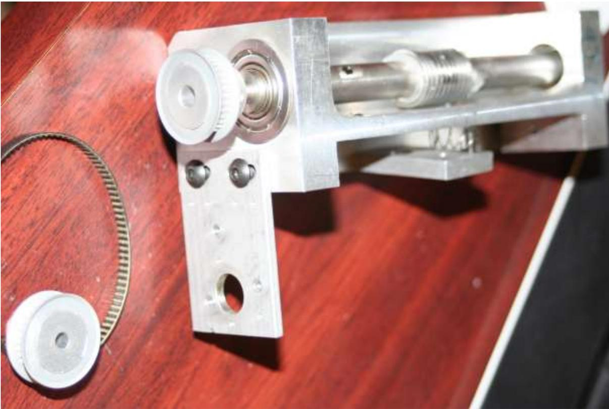
I reinstalled the original Pulleys and belts
