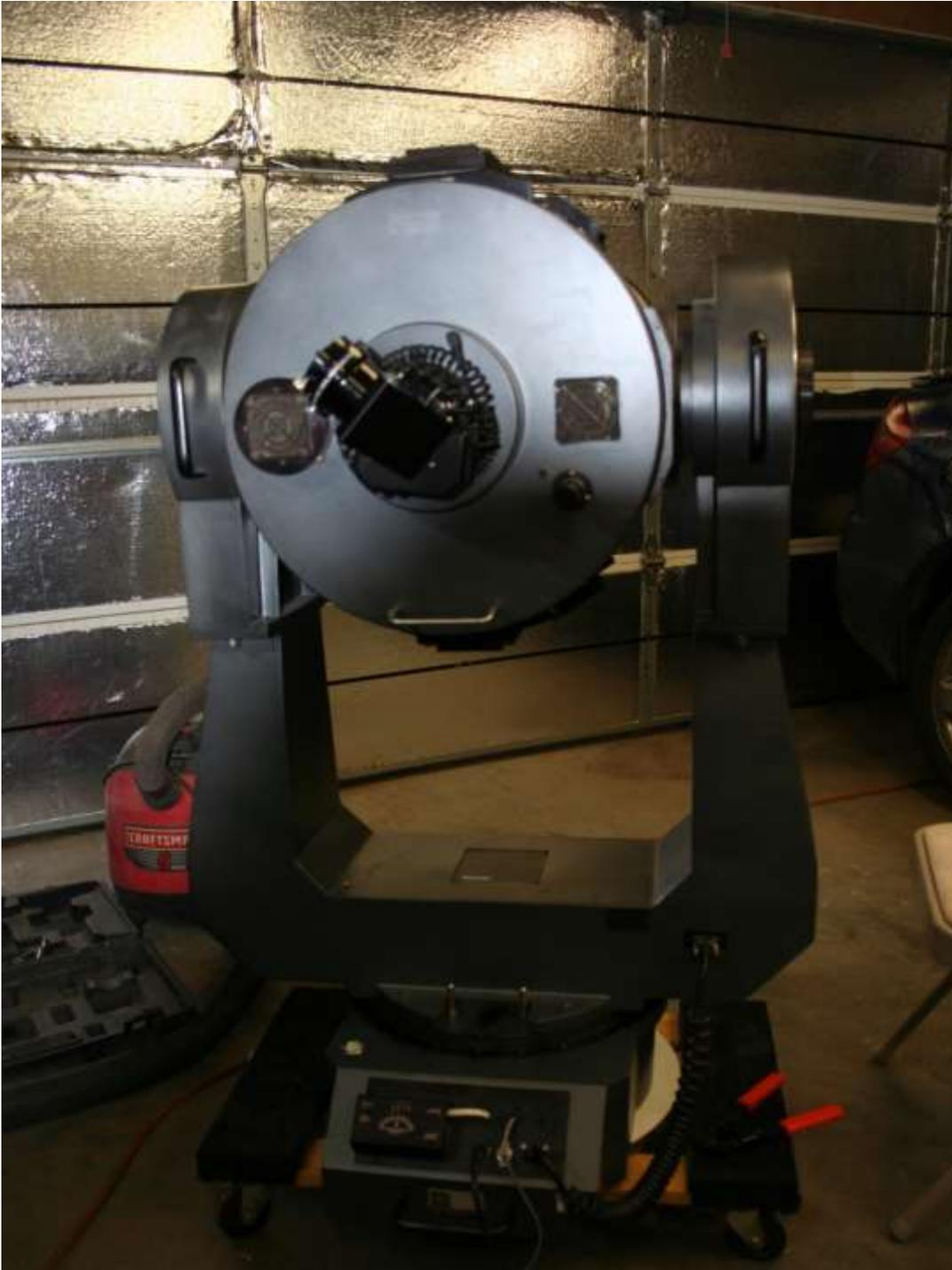
So the scope was again disassembled and the motor assemblies removed and the pulleys and belts were replaced with the new ones I ordered from SDP/SI
